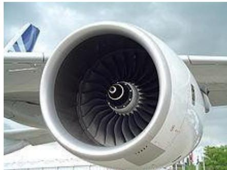
This shows the Rolls-Royce Trent 900 on the prototype on the Airbus A380. This aircraft has four engines.
